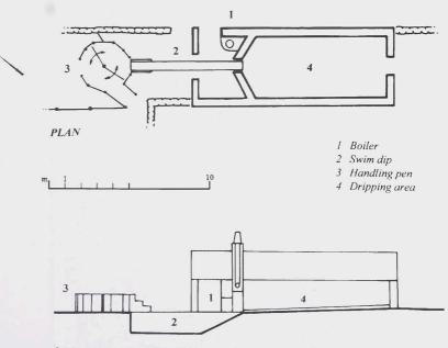
SECTIONAL ELEVATION Detail of item 9 - Covered dipping shed
