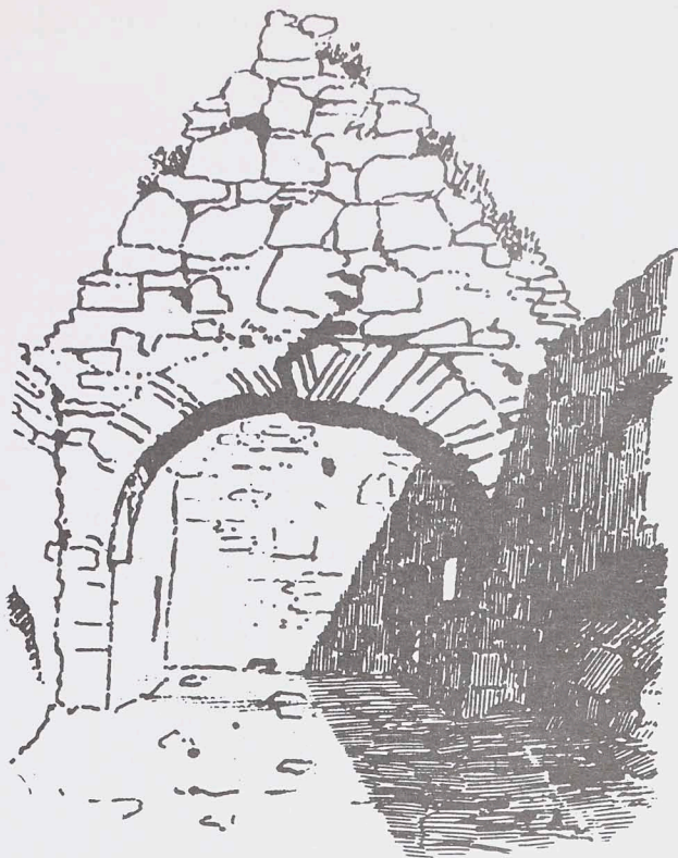
(figure 13) Kirk of Ness, Shetland, the Chancel arch. The detail shown by MacGibbon and Ross (1, p.156, fig. 126) beyond the arch into the chancel has been erased for clarity in showing the setting-out.
