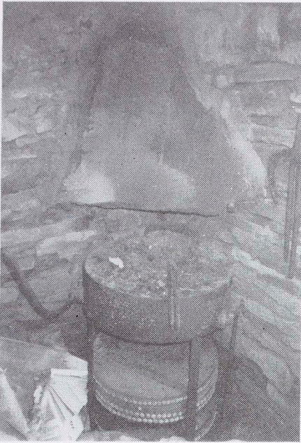
Figure 4 Smithy: portable forge with flagstone chimney.
