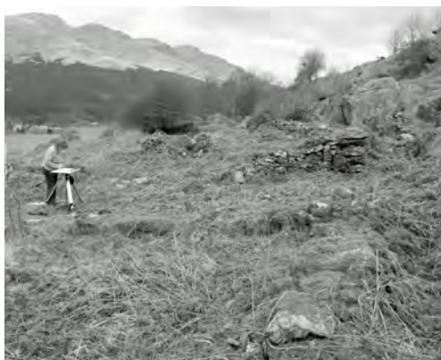
Figure 2. Plane table survey allows SRP volunteers to create detailed plans of abandoned rural settlements. (Crown Copyright: RCAHMS)
